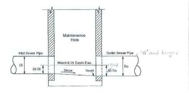
Invert Drop across Maintenance Holes Pipe Sizes 18-inches and Greater Figure F255
