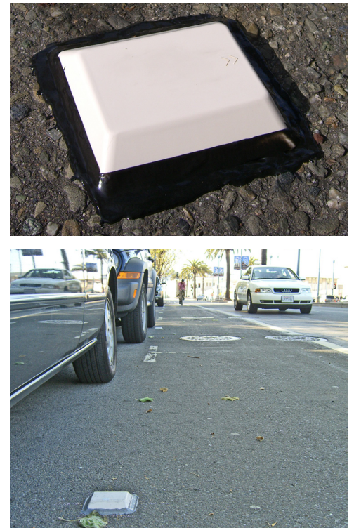
ABOVE: Remote sensors that adhere to the pavement and electromagnetically sense a “parking event” and then wirelessly transmit real-time occupancy data to parking managers. Photos courtesy of Streetline Networks.
