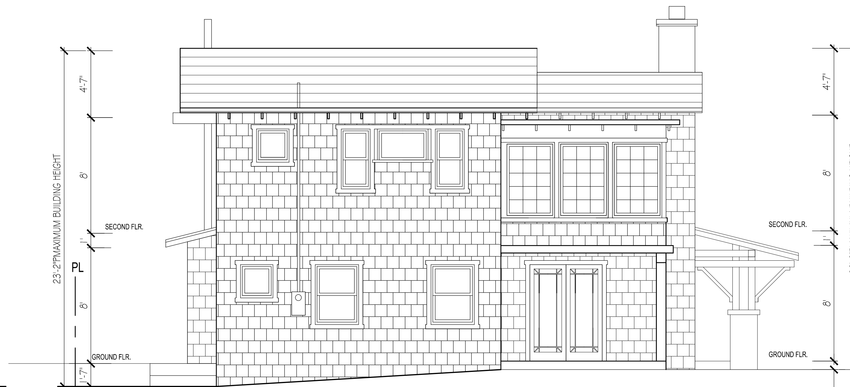
3 EXISTING BUILDING EAST ELEVATION SCALE 1/4"=1'-0"
