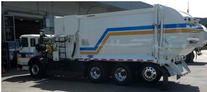
Residents are likely to see this Autocar Wayne Curbtender with 31 cubic yards capacity in residential areas.
