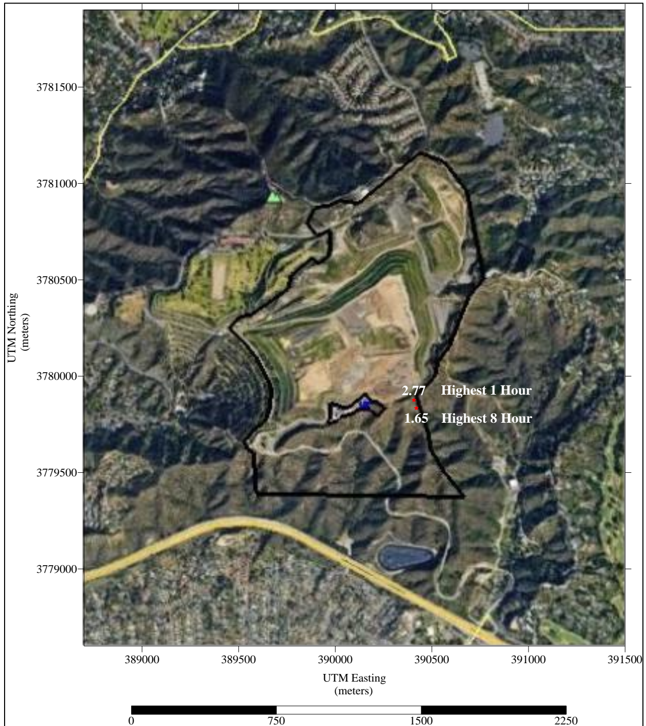
AERMOD Output for 1 st Highest 1-Hourly and 8-Hourly CO Concentrations (in ppm)
