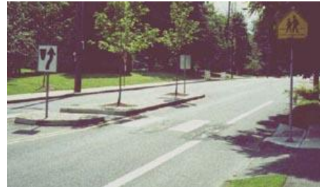
Midblock pedestrian refuge is used to calm traffic near an elementary school in Portland, OR Image from PBOT
