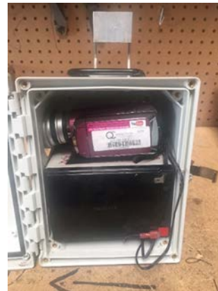
Cameras were placed in protective casings and installed on traffic signal poles to capture screenline data on adjacent intersection legs
