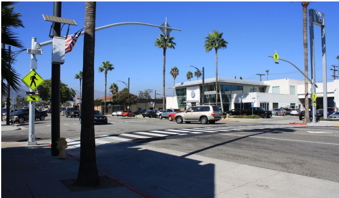
A solar-powered rectangular rapid flashing beacon in Glendale Image from the City of Glendale
