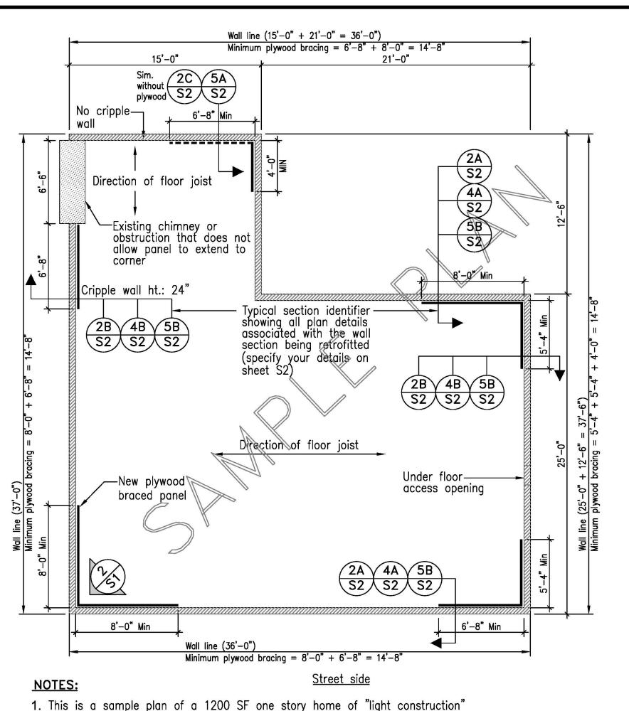
SAMPLE FOUNDATION AND PLYWOOD LAYOUT PLAN
