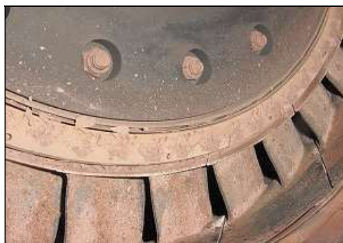
Figure 2. Hard Silicon Deposits on a Turbine Nozzle
