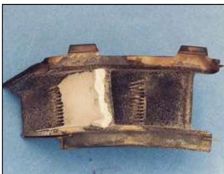
Figure 1. Silicon Deposits on a Turbine Nozzle
