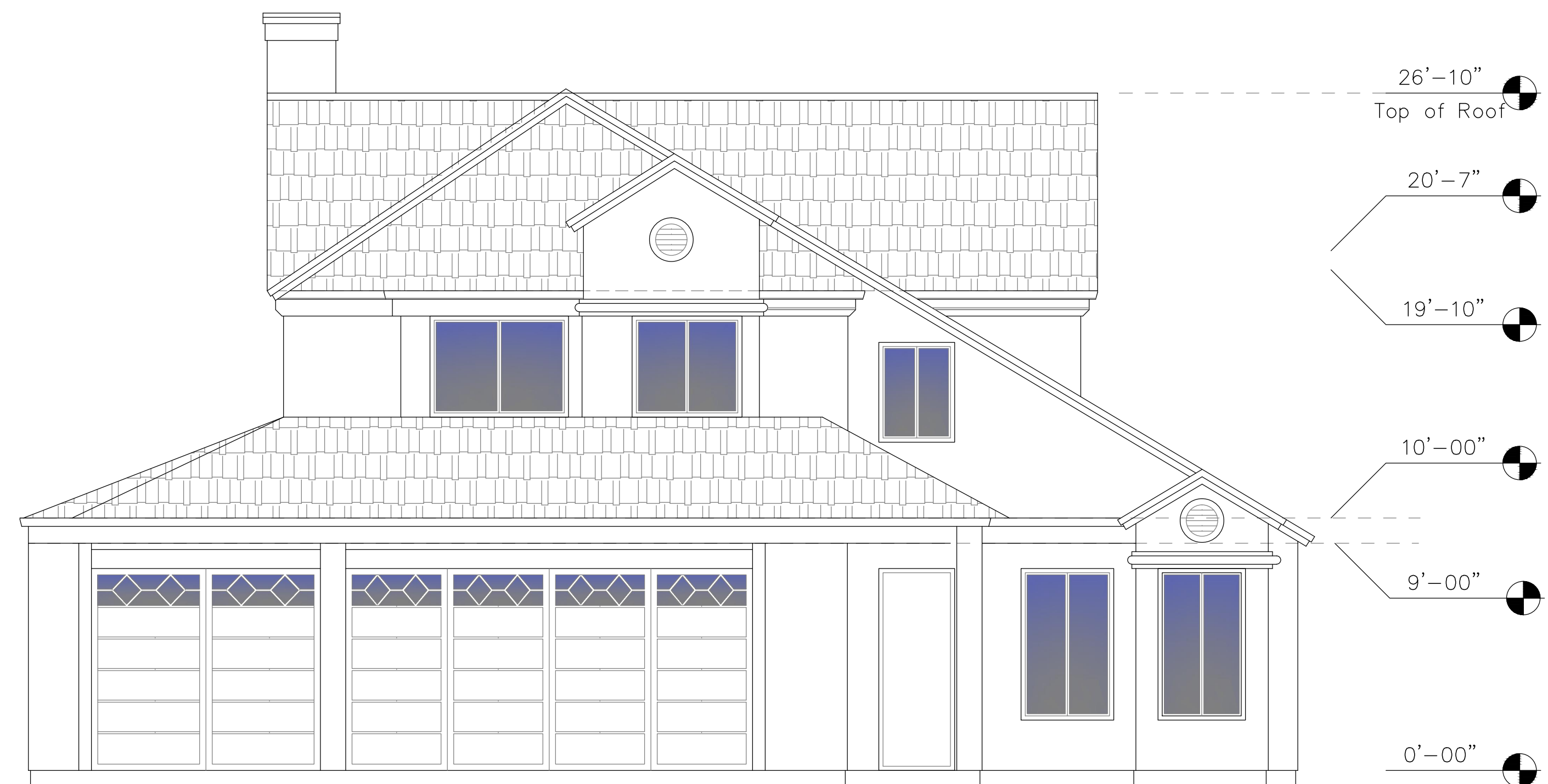
EXISTING NORTH ELEVATION SCALE: 1/4" = 1'-0"
