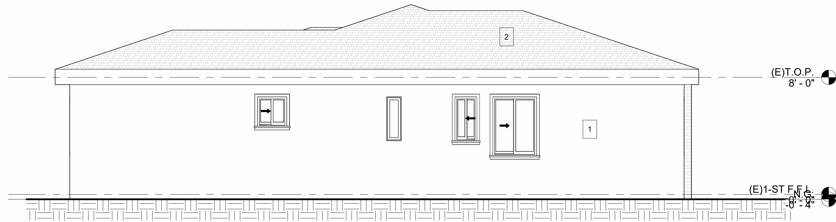
3 EXISTING EAST ELEVATION 1/4" = 1'-0" 0' 2' 4' 8'
